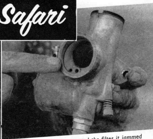
Once the dust had penetrated the filter it jammed open the slides of the carb; this meant frequent stops to clean them.
