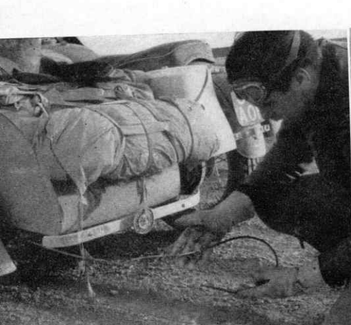
We had to keep up high speeds although this guaranteed damage to our gear and this sidecar brake was torn clean away.
