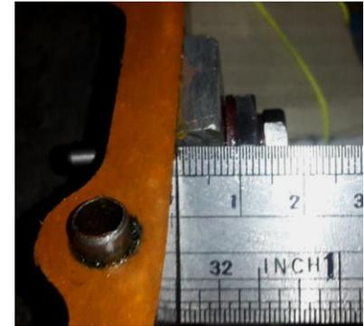
I then removed the oil drain nut which has the built-in level tube, and got a further 160 mls.
